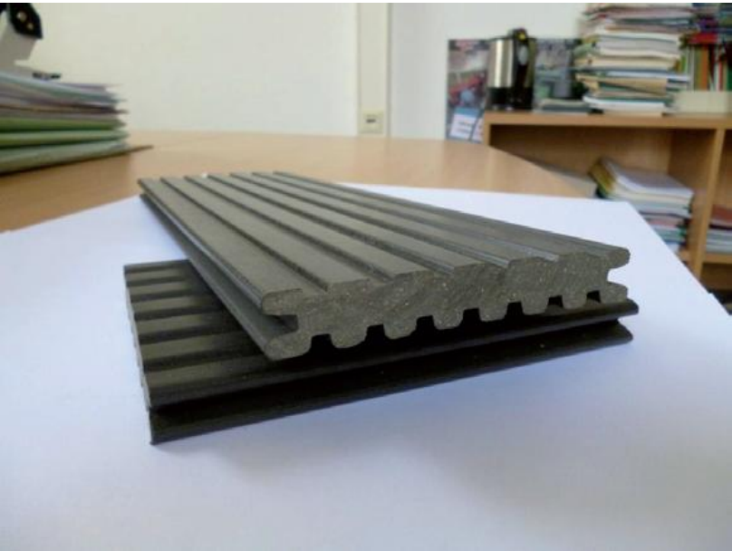
Fig. 4 – Extruded decking boards out of straw / chaff mixture
